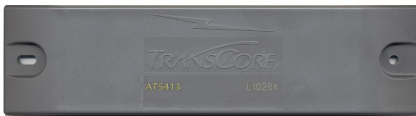
The AT5413 Hardened Rail Tag is a beam-powered, field disturbance device used in 915 MHz radio frequency (RF) band applications. It is packaged in a factory-sealed case, which makes this tag ideal for mounting on railcars, vehicle chassis, intermodal containers, or in any environment requiring a durable, weatherproof tag.
