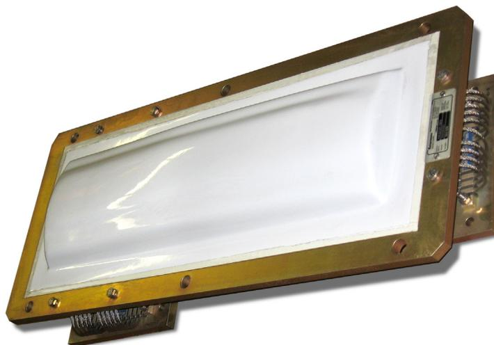
The AA3233-002 Rail Antenna is a rugged 915 MHz antenna specifically designed for the rail industry. The antenna is designed for mounting between track rails. The antenna's optimal performance is achieved when used with a TransCore AT5000-series transportation tag mounted to the underside of rail vehicles. The AA3233-002 operates with a TransCore radio frequency (RF) module.
