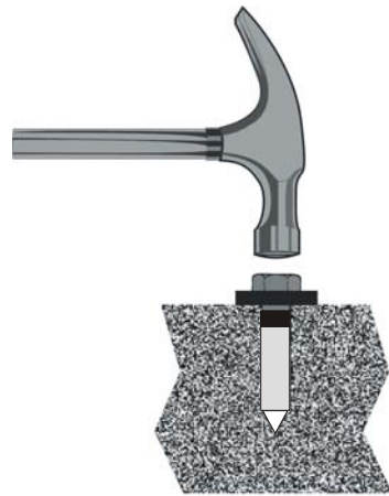
Figure 1-5 Placing Stud Anchor into Hole
