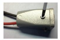
Figure 17 Reassemble and Tighten Set Screws
