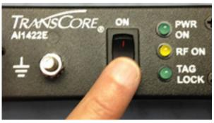
Figure 22 Power the Unit to OFF
