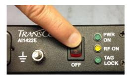
Figure 21 Power the Unit to ON
