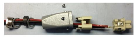
Figure 14 Thread Wires Through Assembly
