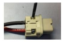
Figure 15 Insert Wires into Pins
