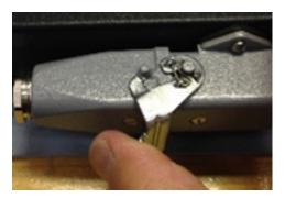
Figure 23 Connector Latch
