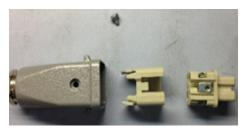
Figure 11 Remove Wire Harness from Insert Clip
