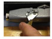
Figure 9 Remove Plug from Receptacle
