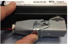
Figure 20 Reinstall Power Connector
