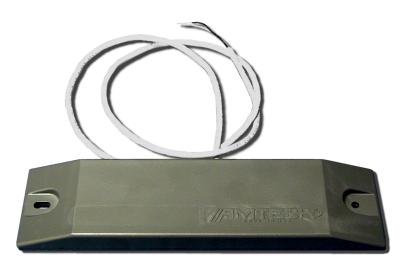
The AT5117 Externally Powered Signal Tag, also called the Signal Transponder, is a single radio-frequency (RF), contact-programmable, externally powered field disturbance device designed for rail traffic monitoring.
