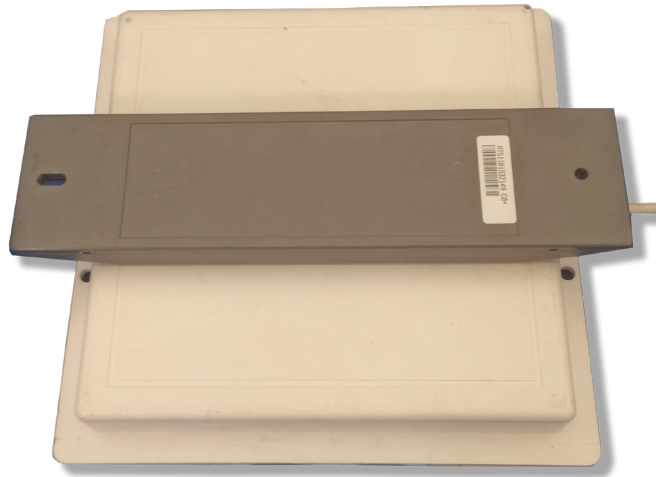
Figure 22 Tag and Antenna Orientation (horizontal polarization)
