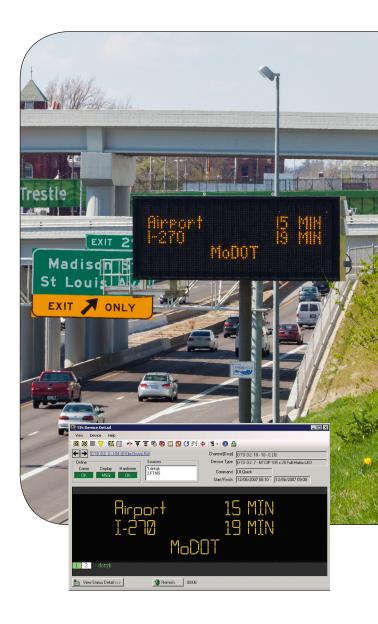
graphical display, customized for the sign type being managed. This allows the user to see the message as it will appear on the sign.
